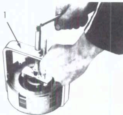
Fig. 125—Use special tool (1) or similar horseshoe shape tool and a press to compress piston return spring during disassembly and reassembly.
