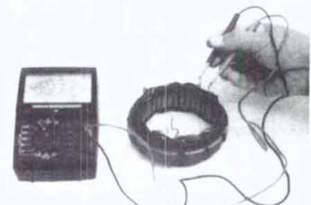
Fig. 77—Check stator coil leads for continuity.
