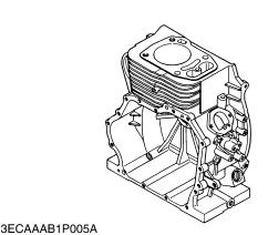
The crank case is made of aluminium die-cast.
