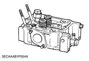
As the cylinder head is subjected to high temperature and high pressure, it is made of special cast iron.
