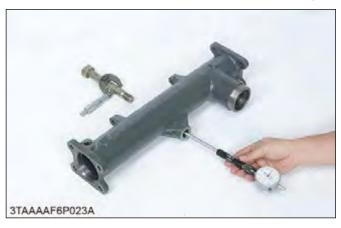
1. Measure the center pin O.D. with an outside micrometer.
