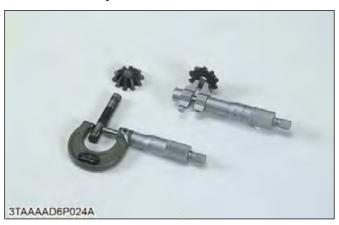
1. Measure the differential pinion shaft O.D.
