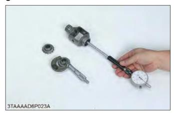
1. Measure the differential side gear boss O.D.
