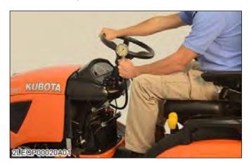
Disconnect the power steering hose L (or R) from steering controller, and set a pressure gauge and hose.
