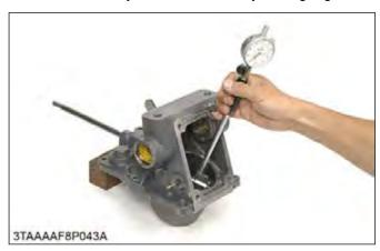
3. If the measurement exceeds the allowable limit, replace the hydraulic cylinder block.
