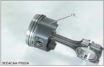
(1) Molybdenum disulfide
