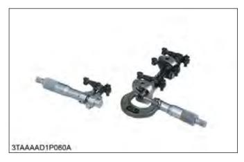
Measure the rocker arm shaft O.D. with an outside micrometer.
