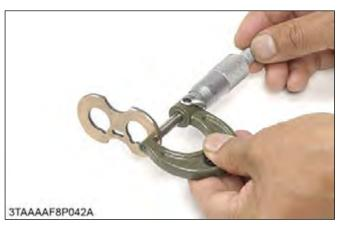
2. If the thickness is less than the allowable limit, replace it.
