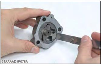
2. If the clearance exceeds the factory specifications, replace the oil pump rotor assembly.
