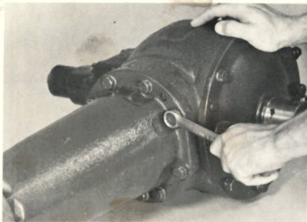
Install the axle housing to the differential assembly.
