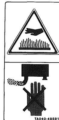
(6) Part No. TA040-4958-1 Do not touch hot surface like muffler, etc.
