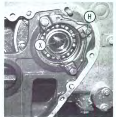
Fig. 106—To remove differential carrier bearing housings, remove three retaining screws (X) and thread two jack screws in holes (H).
