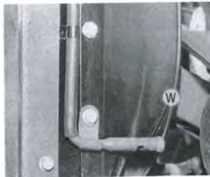
Fig. 72—Whistle (W) on coolant overflow pipe warns of overheating.
