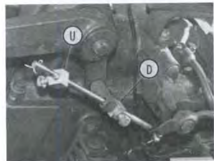
Fig. 133—View of rockshaft linkage rod used on Model L210, showing transport stop (U) and adjustable depth stop (D).
