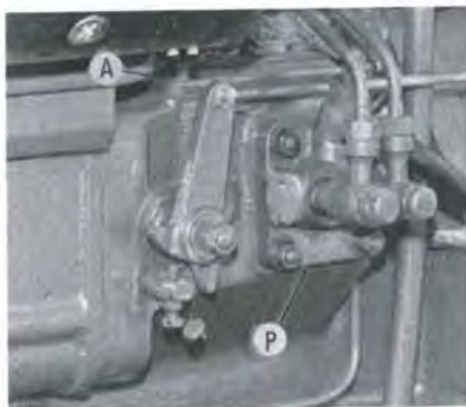
Fig. 32—To remove camshaft on Model L210, first remove access cover (A) and unhook and remove injection pump (P).
