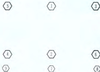
Fig. 8—Cylinder head tightening sequence to be used on Model L210. Refer to paragraph 12 for tightening torques.
