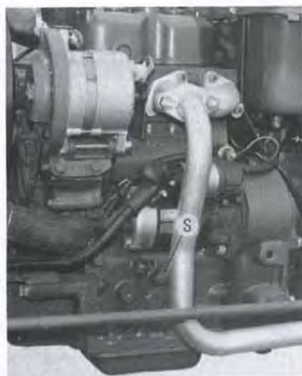
Fig. 38—On Model L175, center bearing housing is positioned by dowel screw (S).
