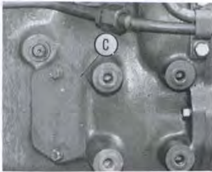
Fig. 85 - Clutch finger height can be adjusted by removing access cover (C).
