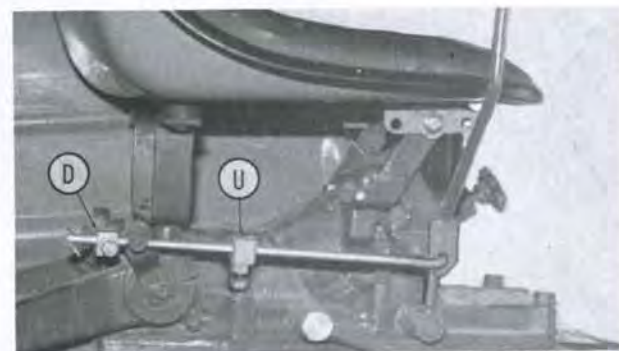
Fig. 131—View of rockshaft linkage rod used on Models L175, L225 and L225DT. Transport stop (U) is permanently set for most jobs; depth stop (D) is adjusted to required working depth.
