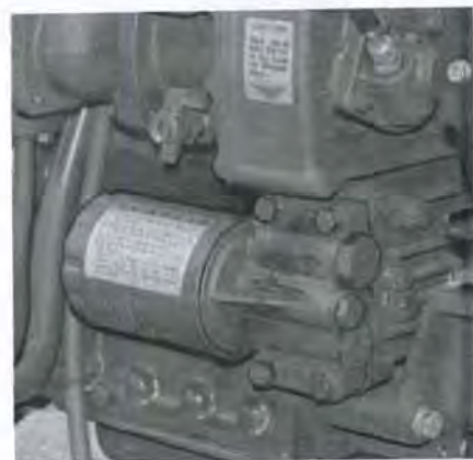
Fig. 45—View of installed relief valve and filter housing of type used on most units.
