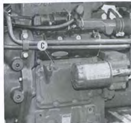
Fig. 33—On Model L210, remove crankcase side cover (C) for access to connecting rod caps and bearings.
