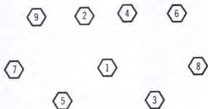
Fig. 10—Cylinder head tightening sequence to be used on Model L260. Recommended tightening torque is 170-184 N·m (125-135 ft.-lbs.).
