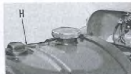
Fig. 129—On Model L210, hydraulic fluid reservoir is built into front of fuel tank as shown at (H).
