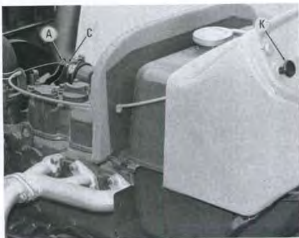
Fig. 11—View of compression release actuating mechanism used on Models L175, L225 and L225DT. Model L210 is similar.
