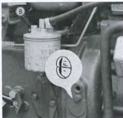
Fig. 51—View of flywheel timing window on Models L175, L225 and L225DT. Inset shows timing marks aligned for number 1 piston firing position. Bleed screw (B) on filter housing is also shown.
