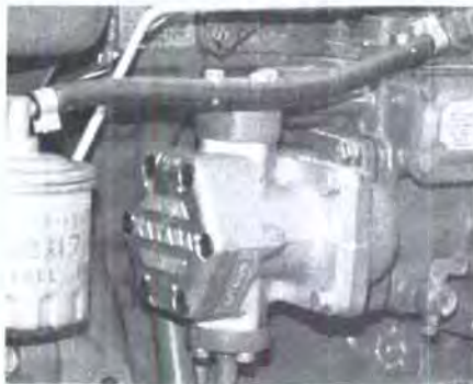
Fig. 135—On Models L175, L225 and L225DT, hydraulic system pump is mounted on right side of cylinder block as shown.
