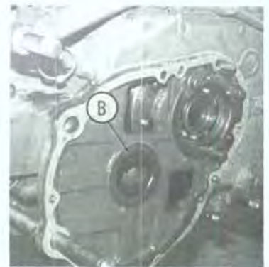
Fig. 117—On Models L175, L225 and L225DT, rear axle inner bearing runs in bore (B) in rear axle center housing.
