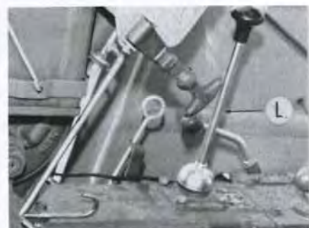
Fig. 98—Before separating Model L210 tractor between clutch housing and transmission, unbolt and lift off shift lever (L).
