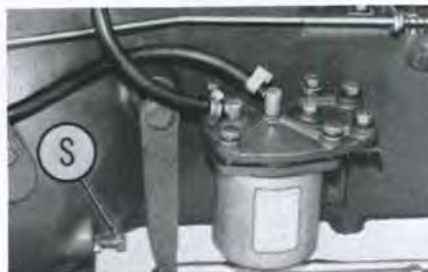
Fig. 87 - On Model L210, stop screw (S) should be adjusted to stop pedal movement just below full disengagement point (F - Fig. 86).
