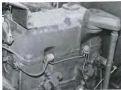
Fig. 71—Right side view of Model L210 engine showing series connected glow plugs. On other models, glow plugs are parallel.
