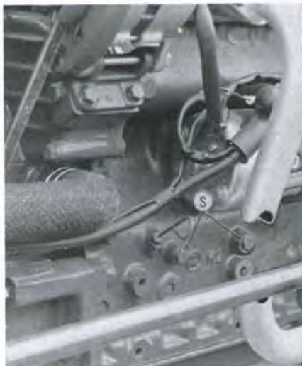
Fig. 39—On Models L225 and L225DT, the two intermediate bearing housings are positioned by dowel screws (S).
