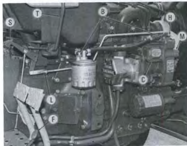
Fig. 53—Right side view of Model L175 tractor showing throttle linkage and points of adjustment or service. Models L225 and L225DT are similar.
