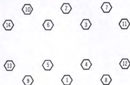
Fig. 9—On Models L225 and L225DT tighten cylinder head cap screws and stud nuts in sequence shown. Recommended tightening torque is 75-82 N·m (55-60 ft.-lbs.).
