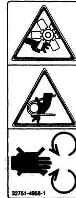
⑥ Part No. 32751-4958-1 Stay clear of engine fan and fanbelt.
