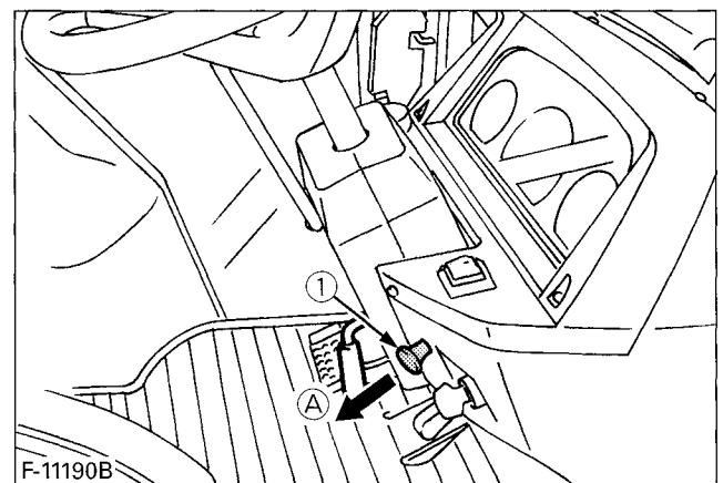
(1) Engine-emergency stop knob
