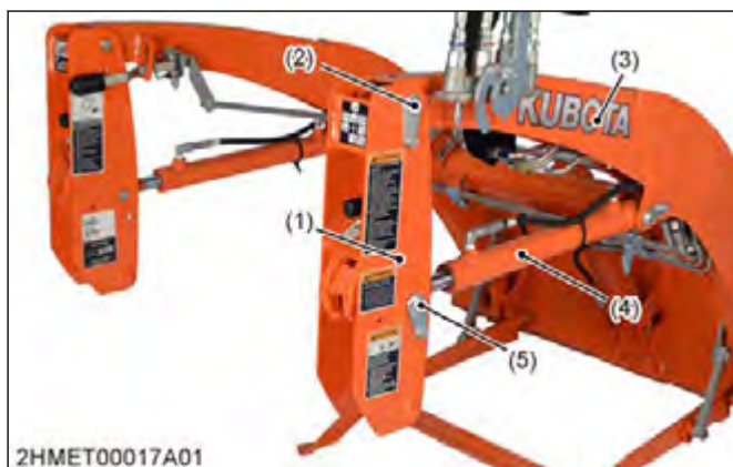
(1) Side frame (4) Boom cylinder (2) Pin (5) Pin (3) Boom assembly
