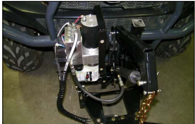
Fig. 13.3—Pump and cover installation
