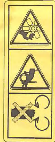
(2) Part No. K2561-6543-1 Stay clear of engine fan and belt.
